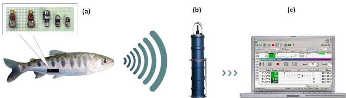
Figure 2. Acoustic telemetry system. As the tagged fish moves through the water the fish identity and sensor data (if available) are relayed by the transmitter (a) at a specific rate to a manual receiver or a set of receivers (b) either submerged or floating on the water (Dagorn *et al.*, 2007). Stored data are collected from receivers and uploaded to a computer (c) for analysis. Image courtesy of [www.biosonicstelemetry.com](http://www.biosonicstelemetry.com).
